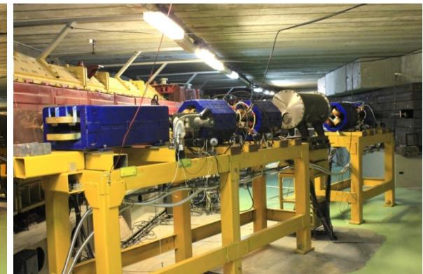
Front-end section of BTL #25 (18 m, 3D, 4Q, 2DCV)
