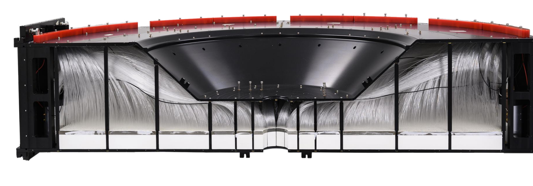
Attachment of optical fibers to scintillator
