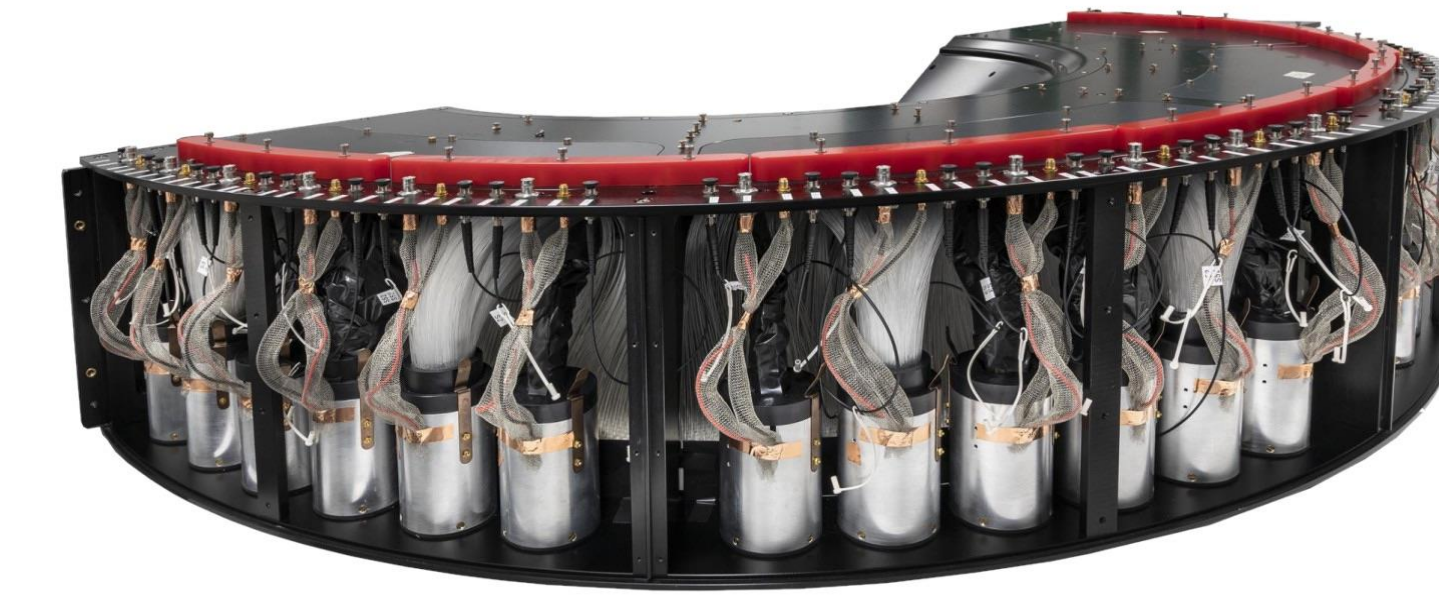
FV0 PMTs and fiber bundles arrangement
