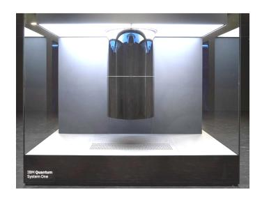
IBM Q System One, a quantum computer with 20 superconducting qubits.
