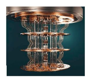
1. An IBM Quantum computer based on superconductiong qubits
