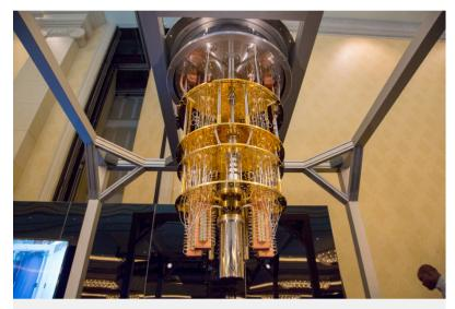
A quantum computer, such as this 50-bit version that IBM demonstrated at the International Consumer Electronics Show in 2018, is capable of solving tasks inaccessible to the most powerful "classic" supercomputer. (Photo: IBM)
