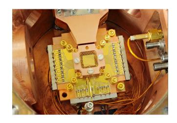
2. Chip ion trap for quantum computing from 2011 at NIST (National Institute of Standard and Technology)
