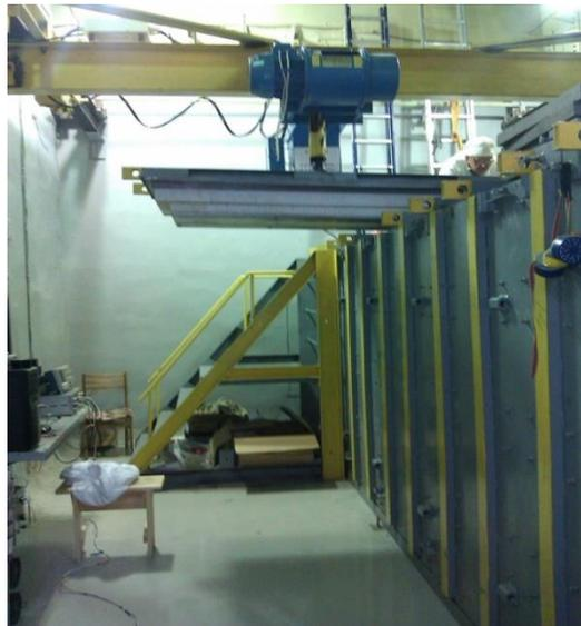
Passive shielding - 60 tons
