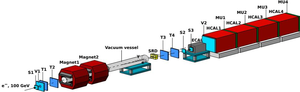
Fig. 2. The schematic illustration of the NA64 detector used for the search for invisible  $A'$  decays produced in the reaction  $eZ \rightarrow eZA'$  in the electromagnetic calorimeter.
